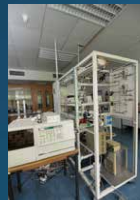
MAT -Micro activity test of FCC catalyts with gas product analysis
