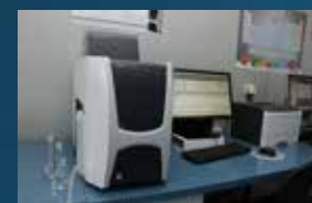
TOC-L+TNM-L – total and dissolved organic carbon, total nitrogen in water
