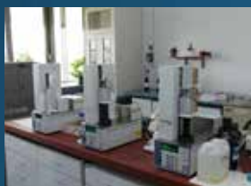
Units for testing of low-temperature properties of petroleum products - filterability, cloud point, pour point
