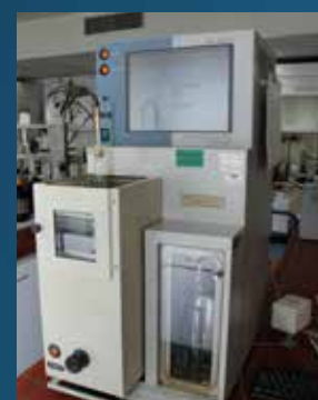
Distillation Unit - testing of distillation characteristics of petroleum products
