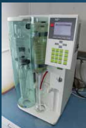
Distillation Unit - distillation of water samples, oil and petroleum fractions after decomposition - the determination of nitrogen by the Kjeldahl method
