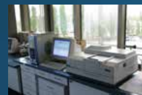
UV/VIS spectrophotometer – anionic and cationic detergents, iron (bivalent), determination of plant available phosphorus from the soil
