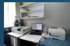
AMA Mercury Analyser – mercury in water, solid and organic samples
