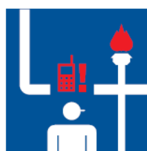
Ensure safe atmosphere in fire box before igniting the burners
