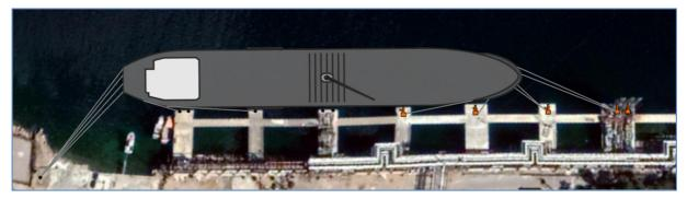
12 mooring lines (4 head/stern lines and 2 forward/aft spring lines)
